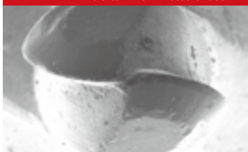
IX-EPDB-TH3 120分加工後 IX-EPDB-TH3 after 120 minutes of use
